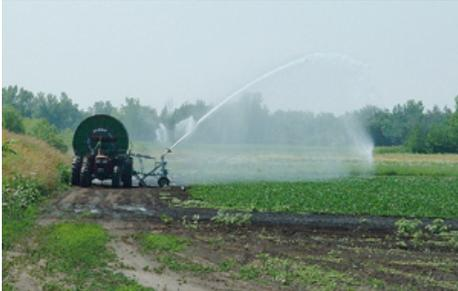
An unattended-operation water reel irrigation unit with automatic shutoff is among the equipment being demonstrated at the August 7-9, 2018 Empire Farm Days. Photo: Kifco
