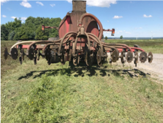
Left: Manure applicator in field; photo Nuhn Industries. Right: Trident 5550 applicator; photo: Monroe Tractor
